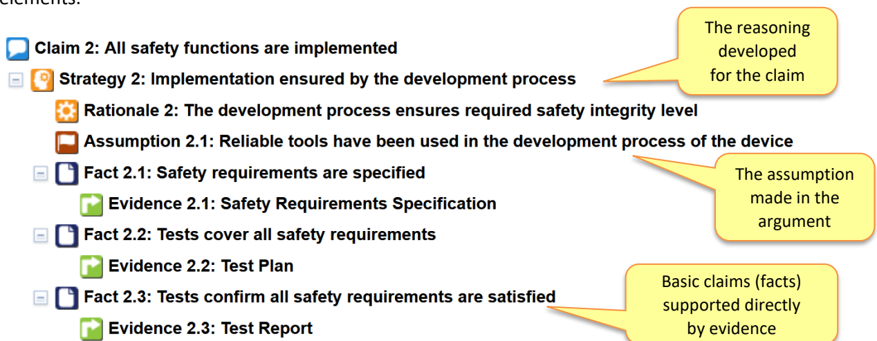
Figure 8. Argument step for implementation of safety functions (hierarchical notation)
