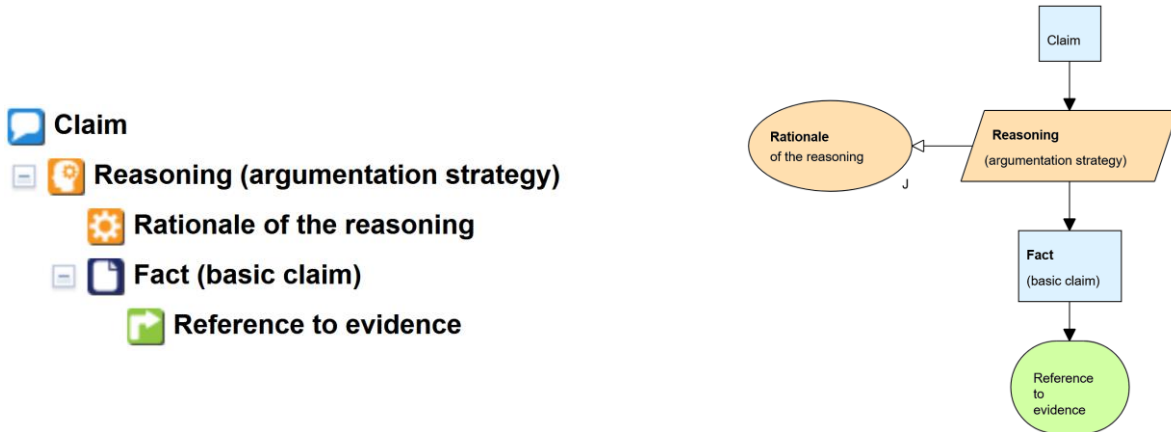
Figure 3. An argument in NOR-STA hierarchical notation (left) and a corresponding GSN diagram (right)
